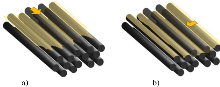
Figure 1.- Two different types of interlaminar crack growth: a) longitudinal, and b) transverse.
